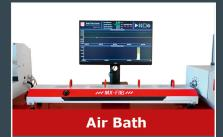
The air bath cools the extruded filament with adjustable airflow, ensuring gradual cooling, dimensional stability, reduced internal stress, and consistent roundness.
