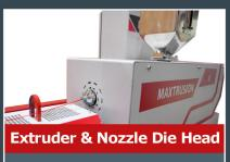
Designed for testing and developing production of standard filaments, with a Die Head Nozzle 1.3: 3 mm.
